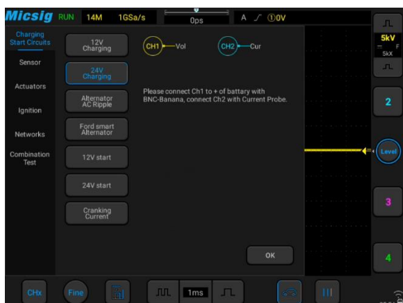
▲ SATO able to test the charging circuit and starting circuit to check whether the car charging /start-up circuit is working normally.
