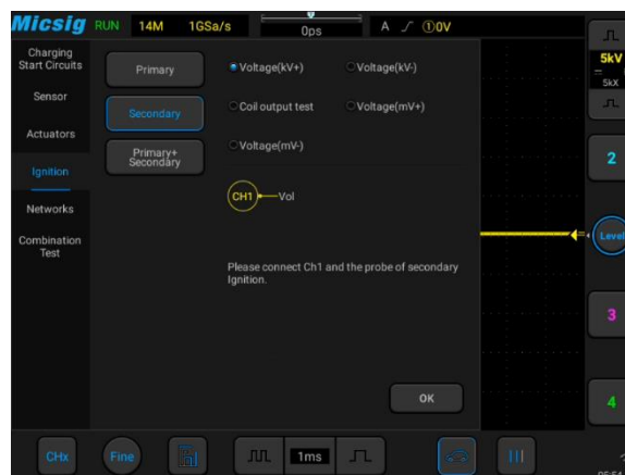
▲ The ignition system of a car is usually composed of primary and secondary coils and spark plugs. SATO can test both Primary and Secondary ignition signals, to find out possible malfunction.
