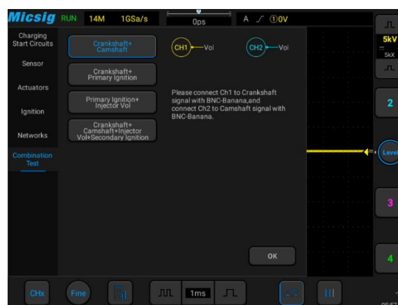
▲ The electronic faults can be complicated, use SATO to perform combination tests, by comparing the collected various waveforms, it helps users judge faults by analyzing the timing and quantitative relationships between waveforms.
